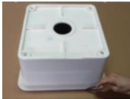
2. Draw a second line the correct distance inside the marked line based on the sink you have. Allow for a 5mm internal overhang.
