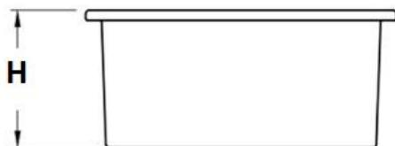
6. Apply some approved flexible watertight silicone to the top of the sink. **DO NOT USE EPOXY OR ANY OTHER SOLID ADHESIVE AS THIS MAY CRACK THE SINK OVERTIME AND WILL VOID THE WARRANTY**, then place the benchtop over the top of the sink. wipe away excess silicone, and leave to cure for 24 hours before use
