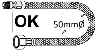
Observe the minimum bend radius of 50mm.
