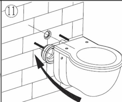
Fit the protective sleeves to the pan bolts.
