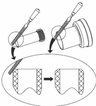
Clean and chamfer cut edge as shown
