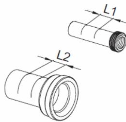
Measure the gaps between the marks on the pipes:
