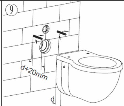
Adjust exposed pan bolt length to  $d+20\text{mm}$
