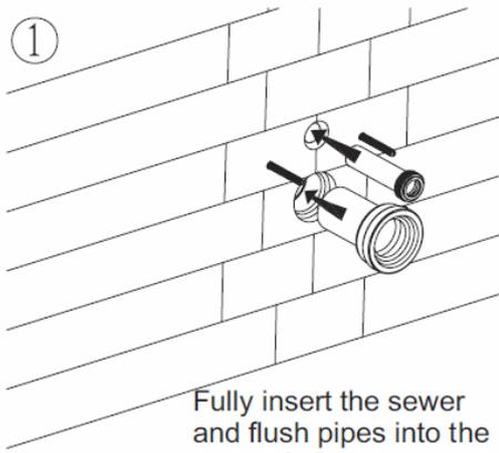
Fully insert the sewer and flush pipes into the concealed connectors
