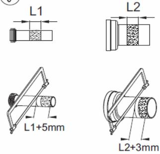
Using L1/L2 dimensions cut the pipes as shown
