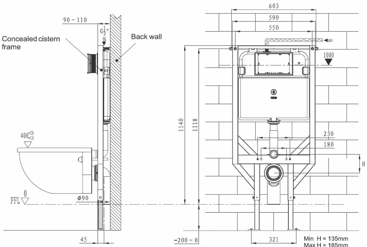
1- Drill holes in the wall and floor then install expansion plugs and screw frame into position.
