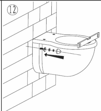
Fit the washers and bolts and tighten securely
