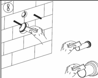
Apply lubricant to the cut pipe end
