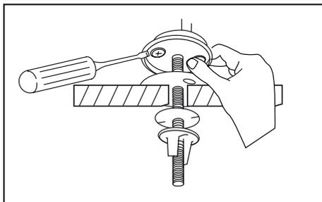
To adjust the seat loosen screw on underside of hinge disc and adjust seat accordingly. Once happy with positioning retighten screw and assemble the seat onto the WC pan.
