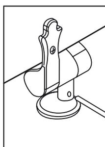
Replace the seat and using the small hex key tighten the grub screws to fully secure the seat into position.
