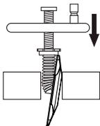
Fix the allen screw into the toggle collar and push through the hole on the top of the toilet pan.
