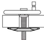
Tighten the allen screw with the allen key provided to secure the top fixing bracket to the pan..
