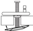
Push the allen screw until the spring loaded bar flips over.
