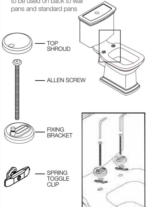
Install the fixing as shown above. Do not tighten fully at this point.
