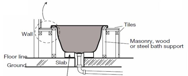
This bath is not self supporting and does require a support at the base via sand/ cement slurry.
