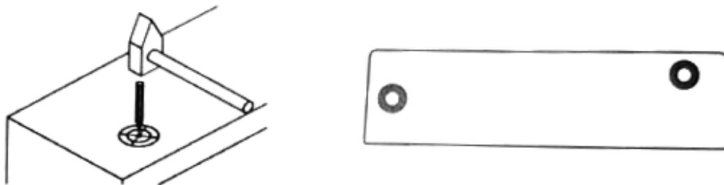
After a few blows the ceramic plug will fall out, leaving a thin layer of ceramic. Remove this with a file. Do not make holes too large.
