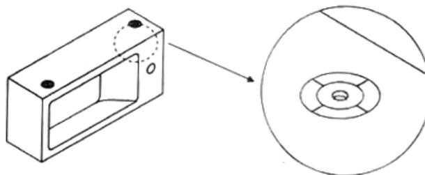
This hole is knocked out by installer. This hole is existing.
